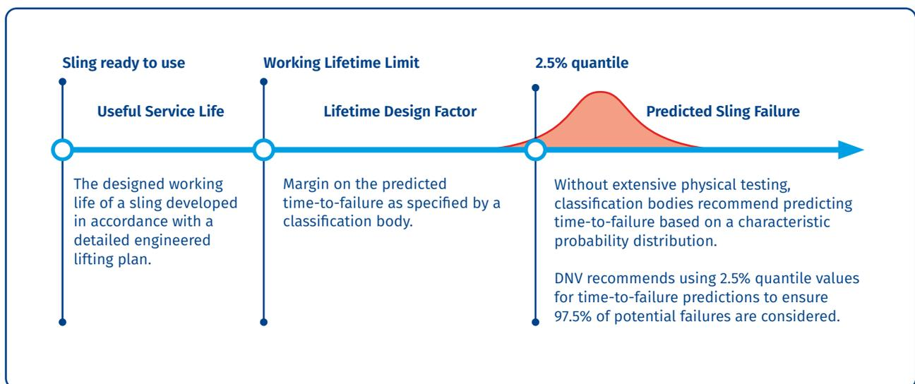
Figure 7: The application of design factors to reliably establish realistic service life criteria from time-to-failure values.
