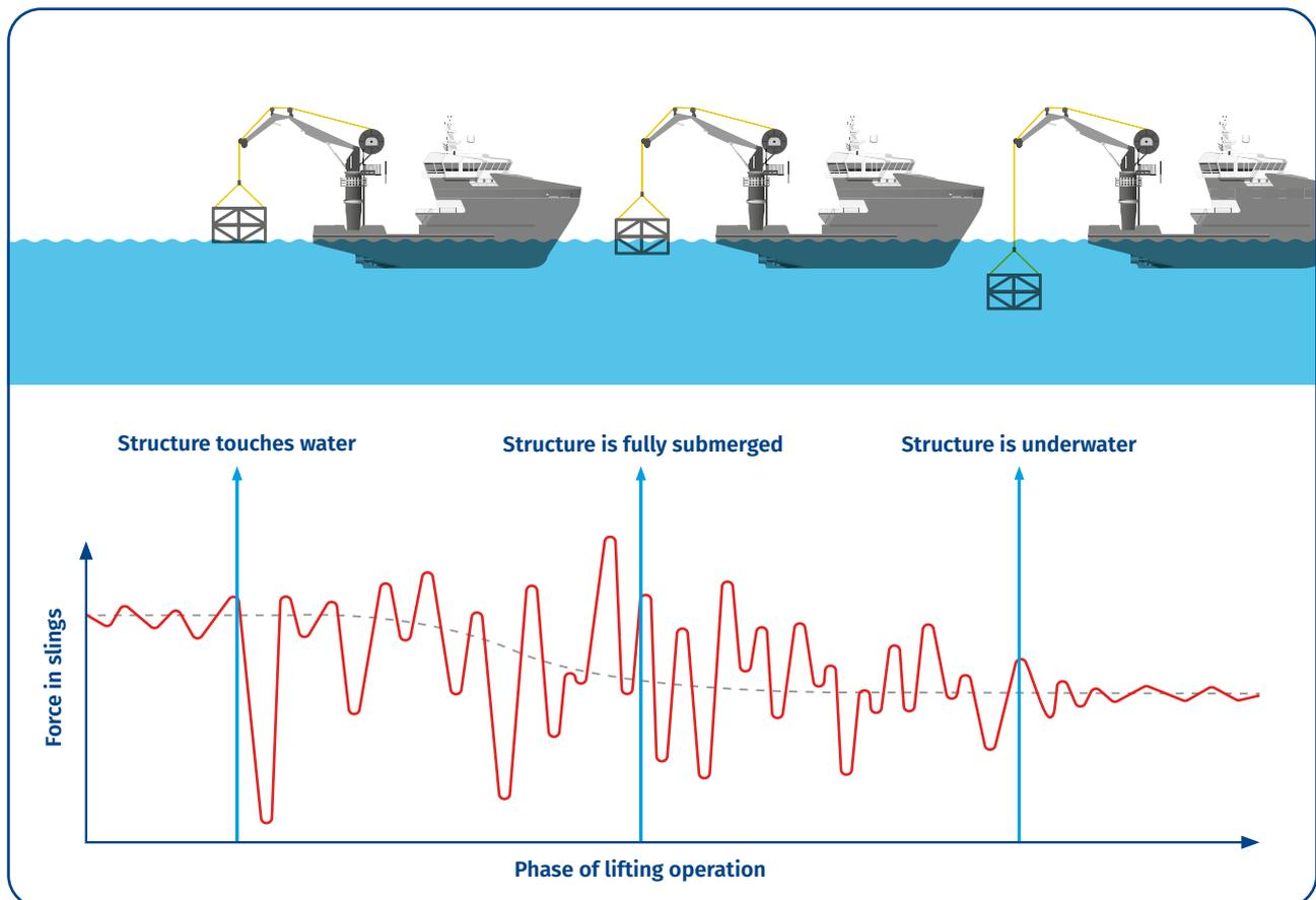
Figure 1: Overview of a typical subsea "ship-to-seabed" lifting operation.
