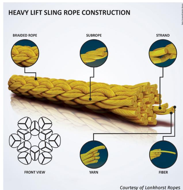
Figure 2: A schematic of the Lanko®Force HL sling with a 12x3 made with Dyneema® SK78 fiber.
