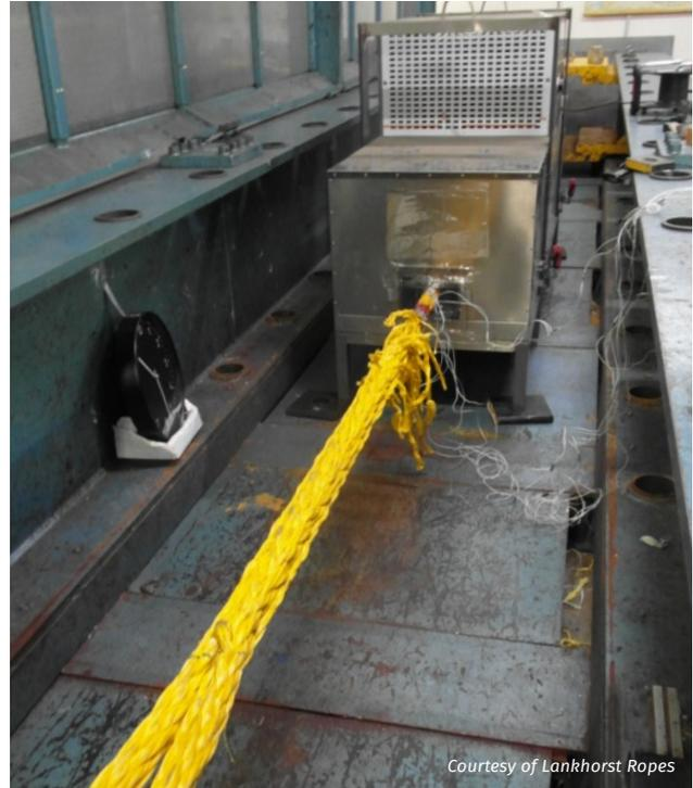
Figure 5: Full-scale fatigue testing set up at Lankhorst Ropes
