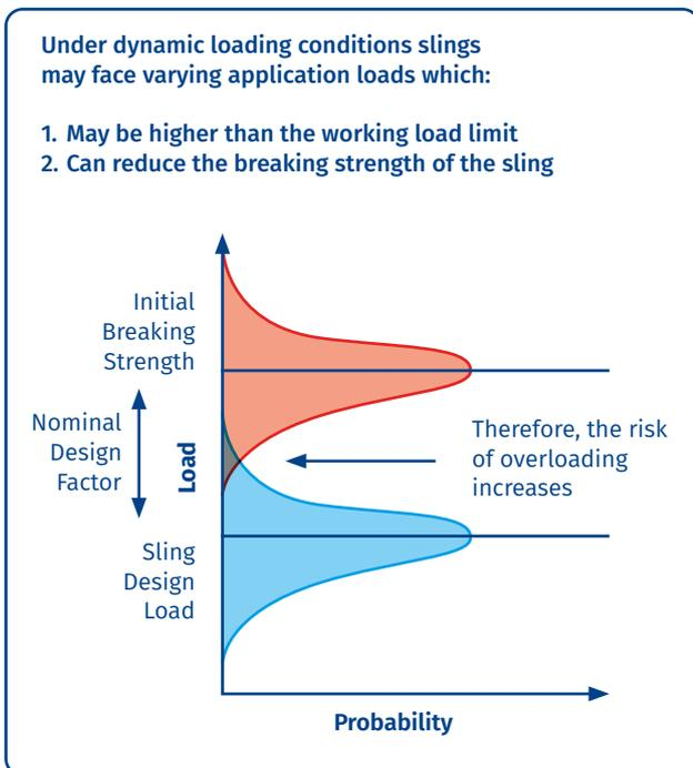
Figure 3: The impact of dynamic loading conditions on reliable sling design.
