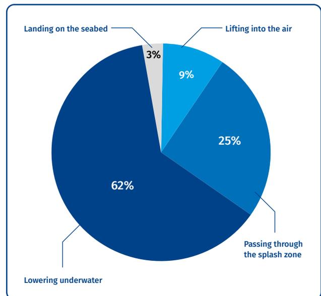
Figure 6: Introduced damage at each stage of the subsea lifting operation as predicted by Avient's Fatigue Performance Model.
