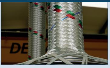
Lankhorst Offshore manufactures deepwater mooring lines based on Cabral® 512 polyester ropes. They utilise high efficiency sub-rope cores laid parallel within a filter system and an outer braided jacket. Each sub-rope is monitored during rope manufacture to ensure all sub-ropes have equal tension and length. Typically, Cabral® ropes include 7 to 18 sub-ropes dependent on the mooring project; each sub-rope is a braided construction, giving a 100% torque free rope.
